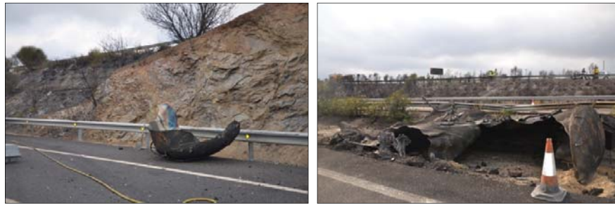
Figure 8. Two main pieces of the tanker after explosion
